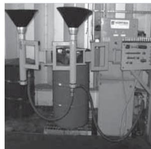
An easy to use system that will quickly drain used engine and transmission oils then pump it away to storage tanks. This avoids moving open tanks or drainers on wheels around the yard to empty them.
